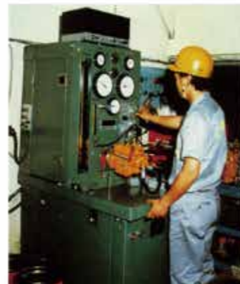
PT Pump Testing
