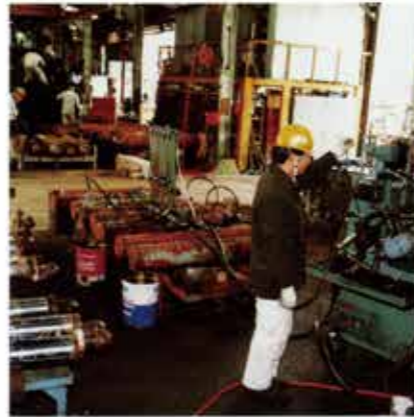
Hydraulic Cylinder Disassembling
